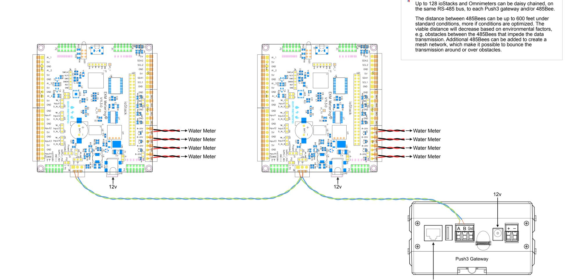
Twisted pair wires. Can be found in CAT5/6 cable. Runs can be up to 4000 feet long. A run could be between an Omnimeter and a 485Bee, between the Push3 and a ioStack, a daisy-chain
