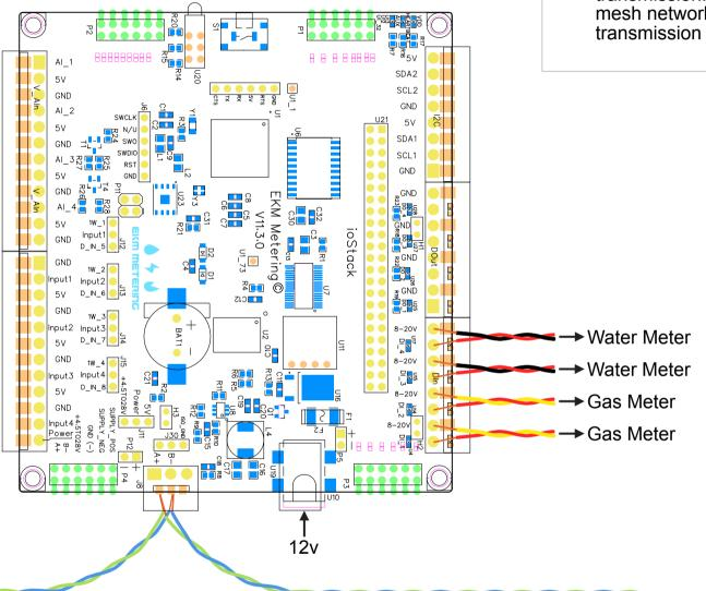
Twisted pair wires. Can be found in CAT5/6 cable. Runs can be up to 4000 feet long. A run could be between an Omnimeter and a 485Bee, between the Push3 and a ioStack, a daisy-chain of Omnimeters and ioStacks, etc.
