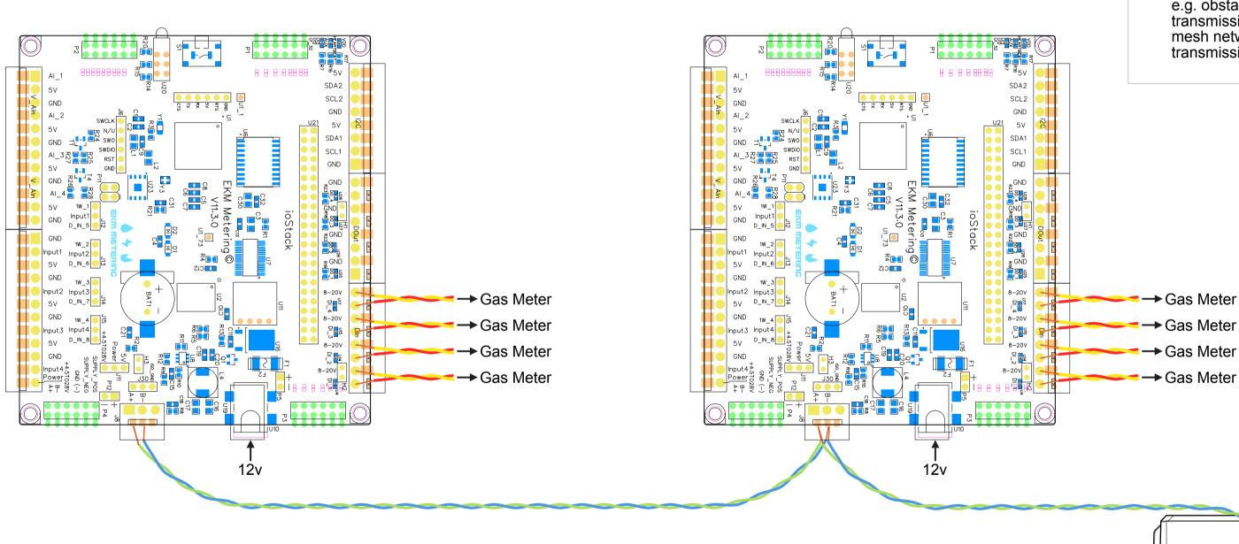
Twisted pair wires. Can be found in CAT5/6 cable. Runs can be up to 4000 feet long. A run could be between an Omnimeter and a 485Bee, between the Push3 and a ioStack, a daisy-chain of Omnimeters and ioStacks, etc.
