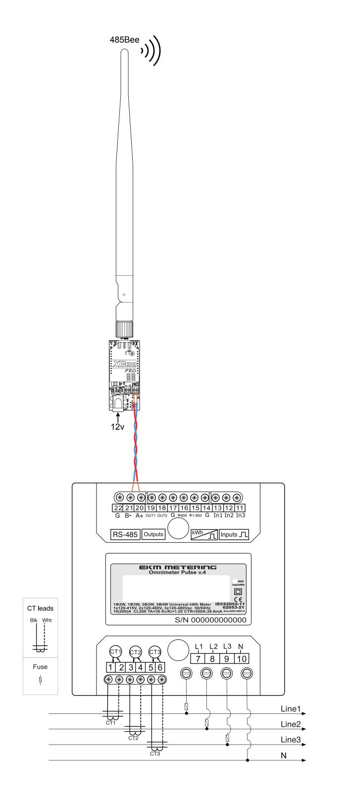
Twisted pair wires. Can be found in CAT5/6 cable. Can be up to 4000 feet long between the Omnimeter and 485Bee, or between the Push3 and 485Bee.
