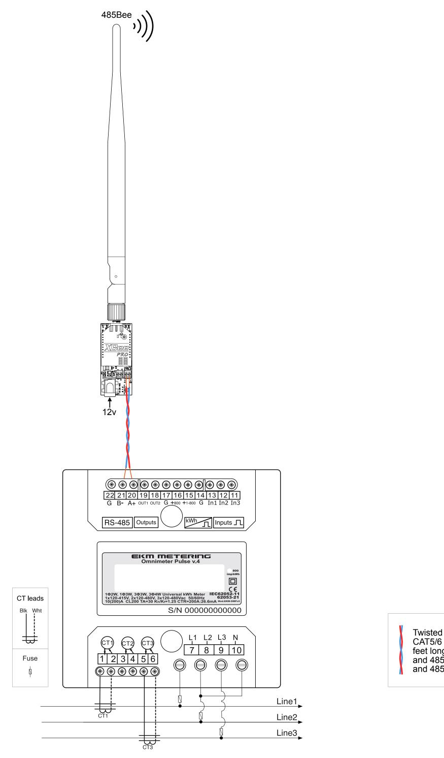
Twisted pair wires. Can be found in CAT5/6 cable. Can be up to 4000 feet long between the Omnimeter and 485Bee, or between the Push3 and 485Bee.
