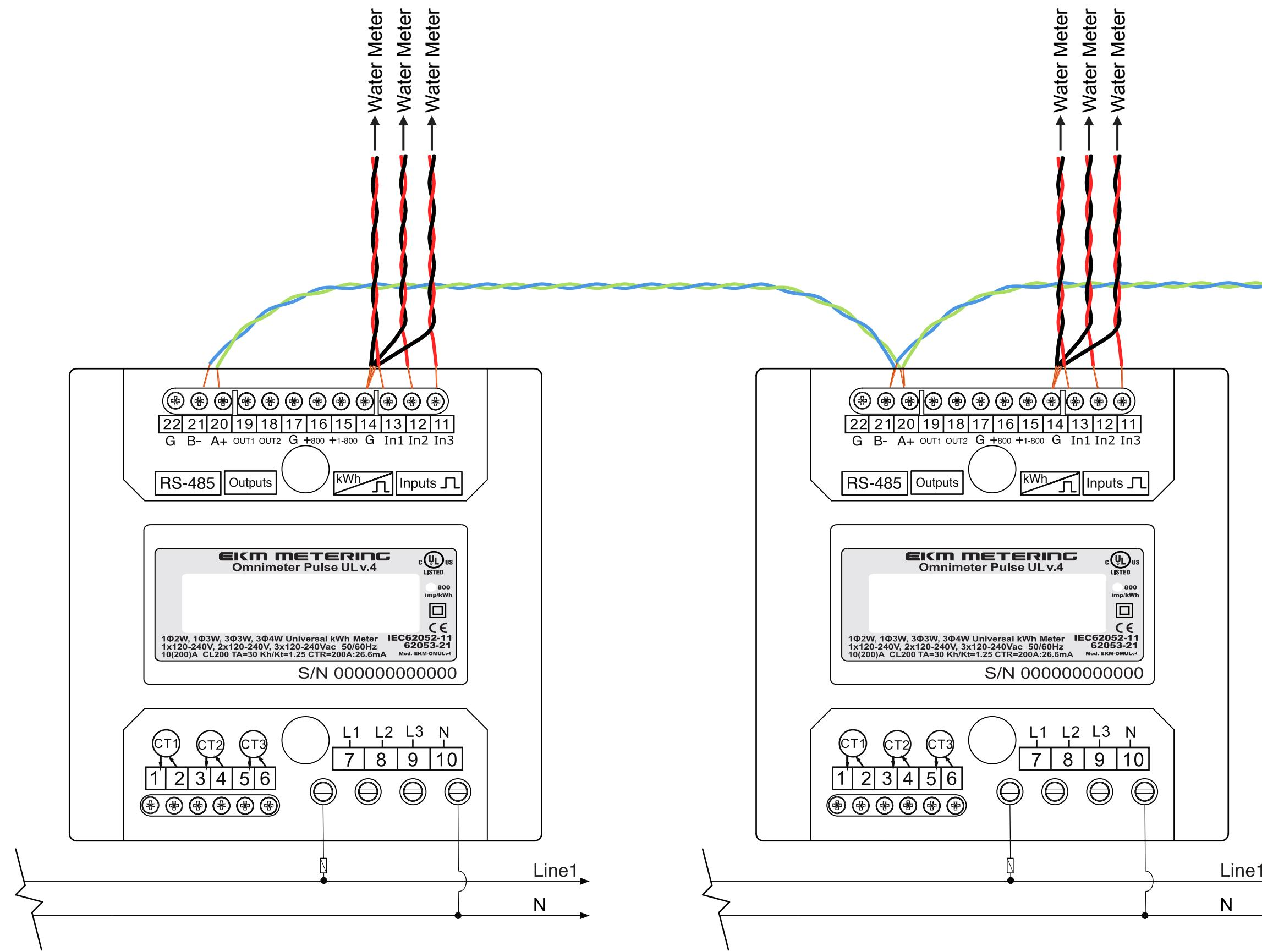
Twisted pair wires. Can be found in CAT5/6 cable. Runs can be up to 4000 feet long. A run could be between an Omnimeter and a 485Bee, between the Push3 and a 485Bee, a daisy chain of Omnimeters, etc.
