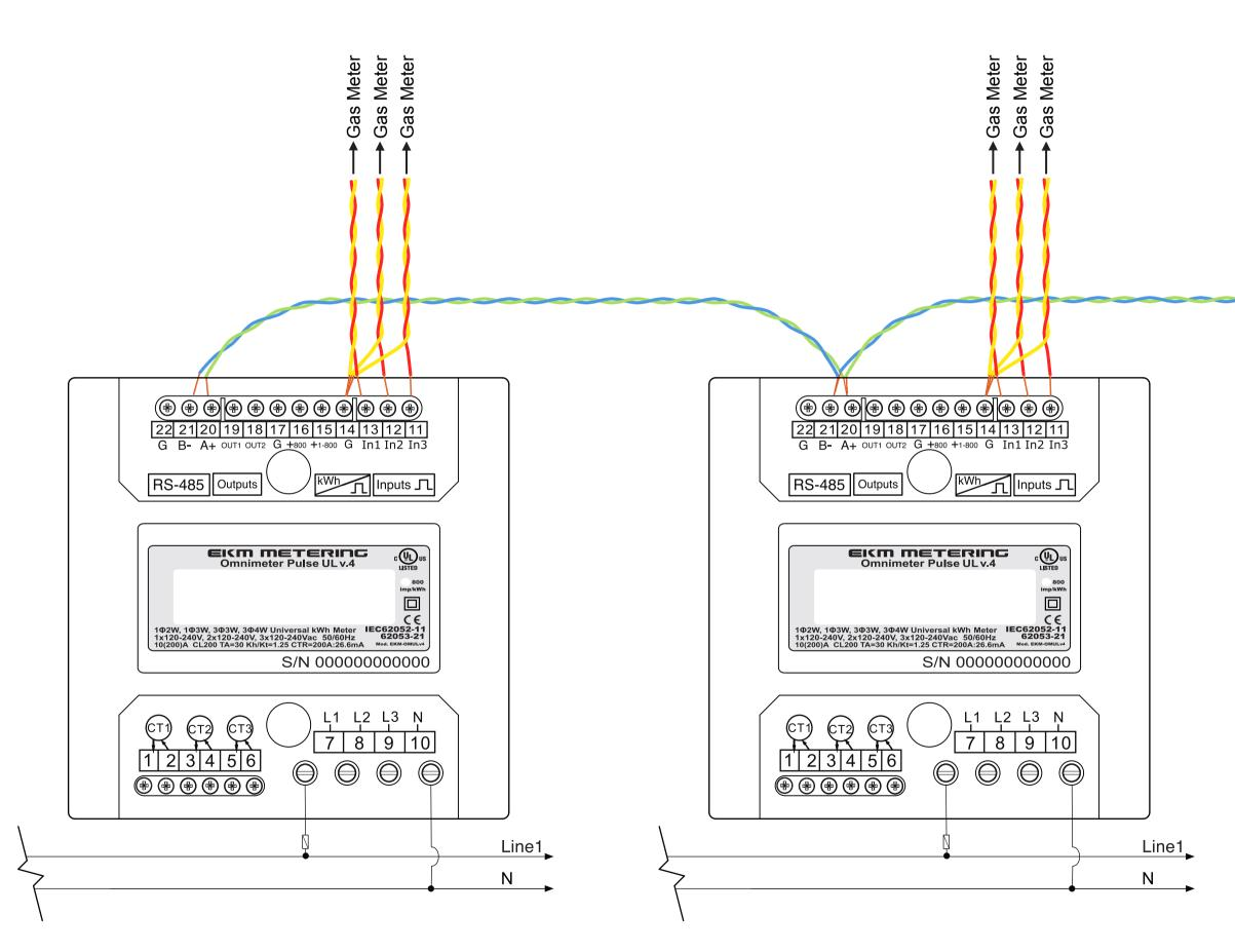
Twisted pair wires. Can be found in CAT5/6 cable. Runs can be up to 4000 feet long. A run could be between an Omnimeter and a 485Bee, between the Push3 and a 485Bee, a daisy chain of Omnimeters, etc.
