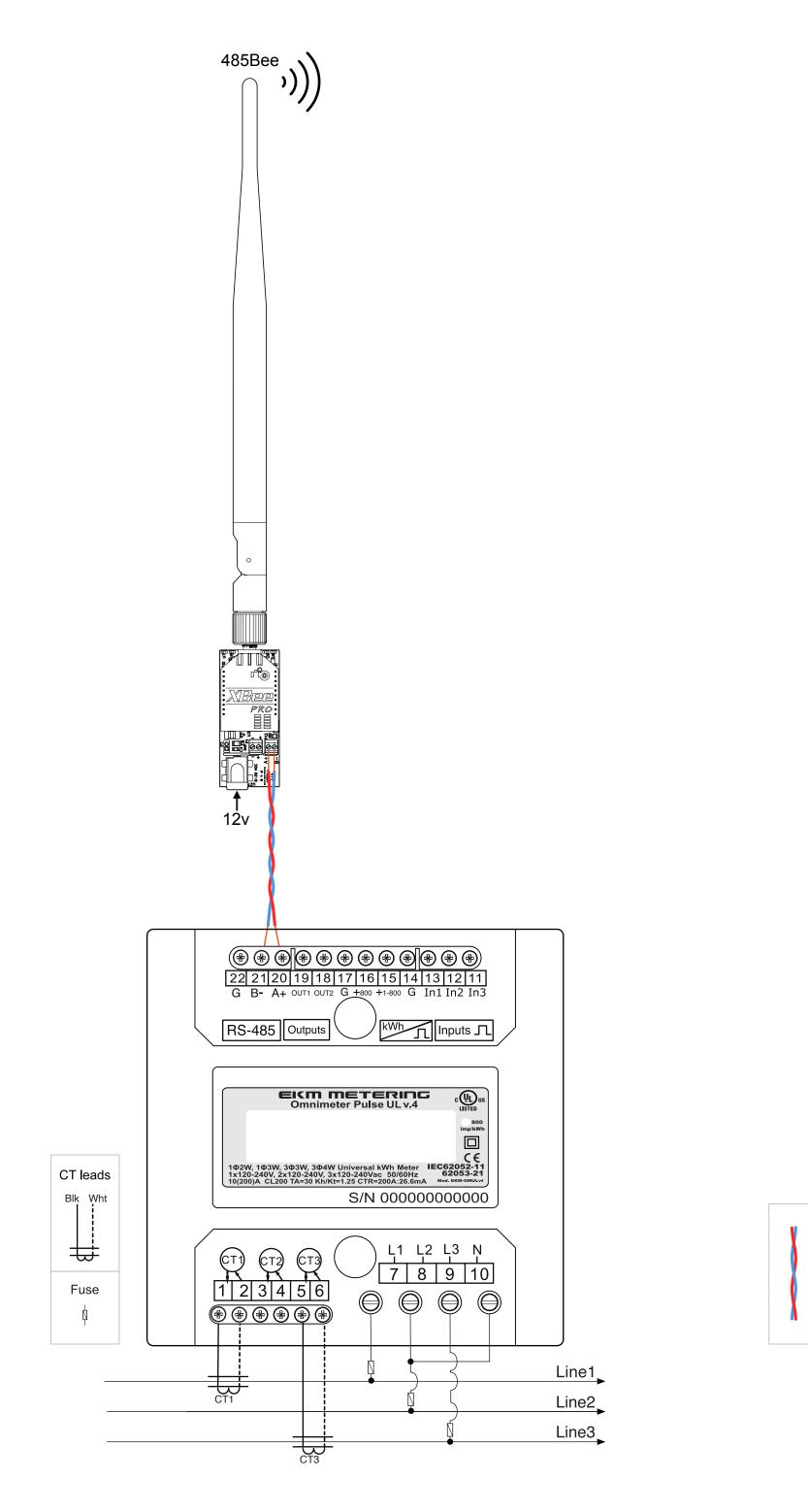
Twisted pair wires. Can be found in CAT5/6 cable. Can be up to 4000 feet long between the Omnimeter and 485Bee, or between the Push3 and 485Bee.
