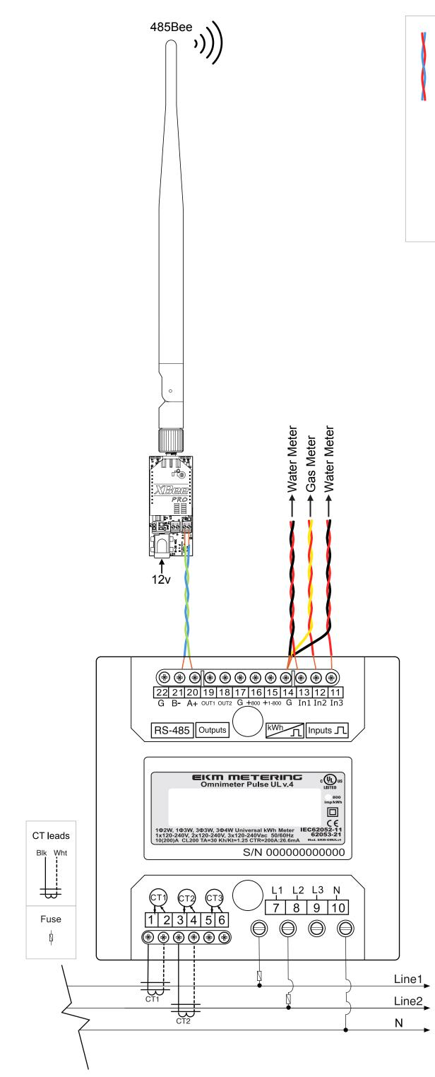
Twisted pair wires. Can be found in CAT5/6 cable. Runs can be up to 4000 feet long. A run could be between an Omnimeter and a 485Bee, between the Push3 and a 485Bee, a daisy chain of Omnimeters, etc.
