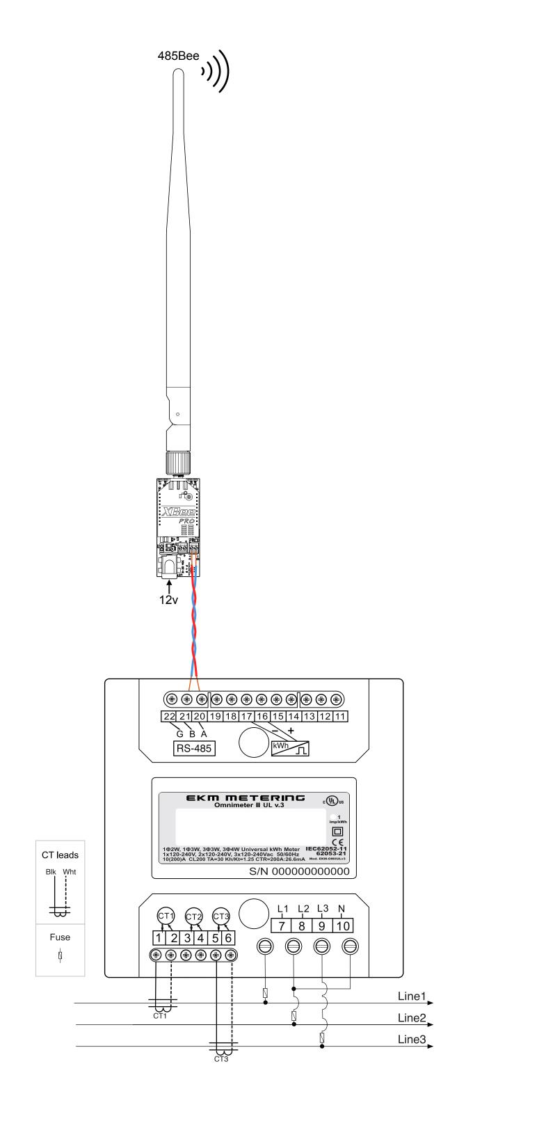
Twisted pair wires. Can be found in CAT5/6 cable. Can be up to 4000 feet long between the Omnimeter and 485Bee, or between the Push3 and 485Bee.
