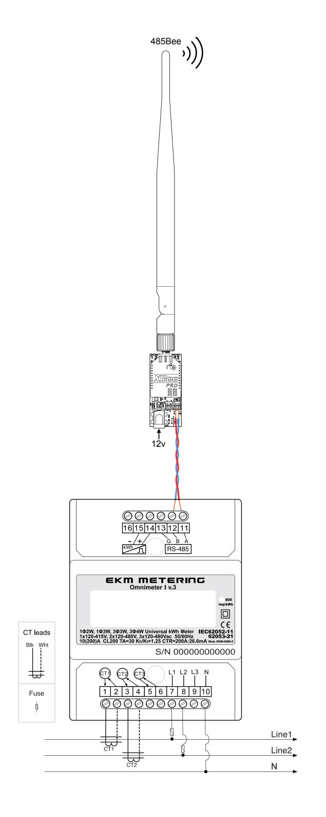
Twisted pair wires. Can be found in CAT5/6 cable. Can be up to 4000 feet long between the Omnimeter and 485Bee, or between the Push3 and 485Bee.
