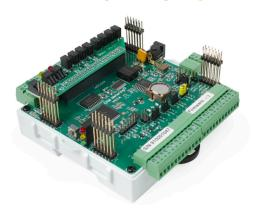
Our EKM-ioStack is a powerful addition to our line of remote readable, affordable metering products. It is not a meter itself, but it does include a lot of features which support or augment your metering system. Fundamentally the ioStack is a sensor input and output hub. It is supported by our EKM Push3 data system via RS485, just like our EKM-Omnimeters.
