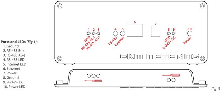
\* Ports 1,2,3,8, and 9 house terminals that are opened or closed through the holes in the top of the Push lid. Insert the screwdriver that came with your EKM Push, into these small holes in order to operate the terminals and connect your wires.
