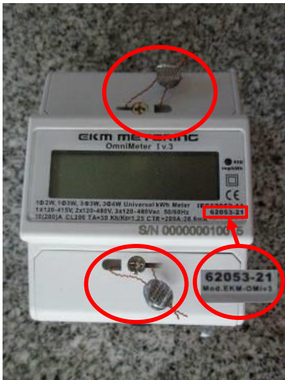
Figure 3. Photos Showing Identification Label and Location of the Wire Security Seals
