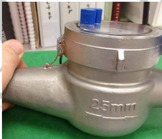
Model SPWM-100-CF Showing Sealing Provisions, Pulse Output Wire Connection and Side View
