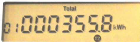
Total kWh (Forward kWh + Reverse kWh)
