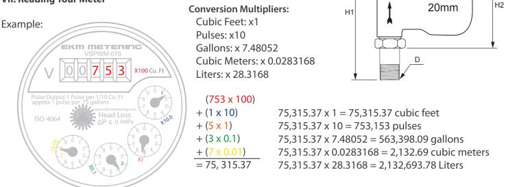
\* Note: Most Utilities in the United States round to the nearest 100 cubic feet. So in this case, only the red portion above, showing 75,300, would be necessary for determining usage.
