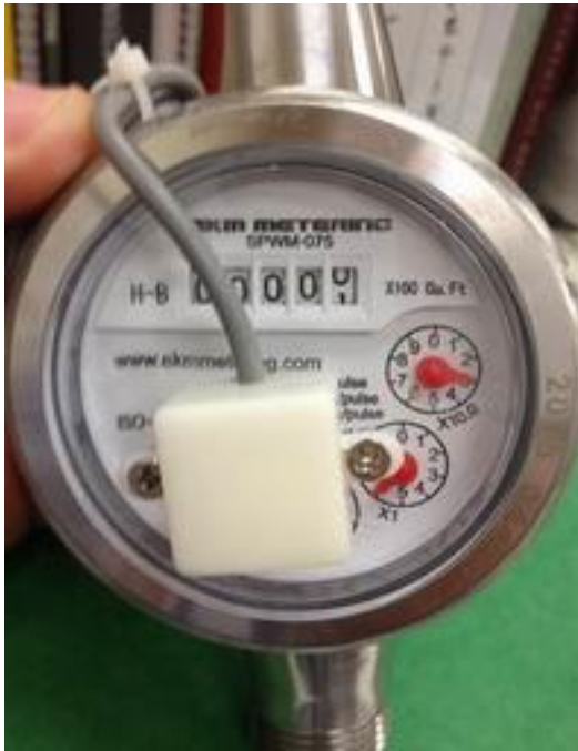
Model SPWM-075-CF Showing Sealing Provisions, Pulse Output Wire Connection and Side View
