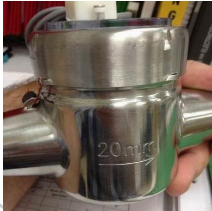
Model SPWM-075-CF Showing Sealing Provisions, Pulse Output Wire Connection and Side View
